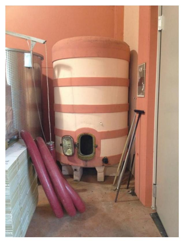
The tank has only ever been washed with hot water, and has accumulated over 40 years of tartaric deposits, which is one of the secrets of Camillo's process (the <u>Baudrys</u> do the same thing with their concrete tanks).
