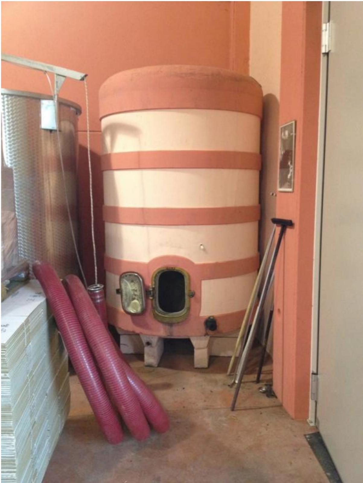
The tank has only ever been washed with hot water, and has accumulated over 40 years of tartaric deposits, which is one of the secrets of Camillo's process (the [Baudrys](#) do the same thing with their concrete tanks).
